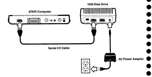
4. Plug one end of the Serial I/O Cable into the jack marked PERIPHERAL on the computer console. Then plug the other end of the cable into one of the two jacks marked I/O CON-NECTORS located on the back of the disk drive.
