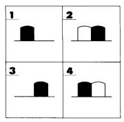
Using a pen or a small screwdriver, set the switches in the window to match the patterns shown here for Drive 1, Drive 2, and so forth. You must always have one drive set as Drive 1.
